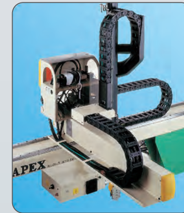
Cable guide protection on all electrical wires and air hoses.
